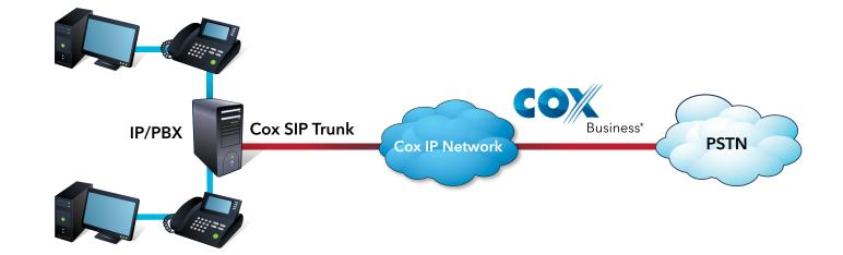
The result is an IP version of Primary Rate Interface (PRI) trunks, the familiar Time Division Multiplexing (TDM) circuit bundles used to feed multiline PBX systems. But instead of using physical trunks with copper wires, SIP Trunking establishes virtual IP channels for real-time communications over an Ethernet connection, be it voice, data, video or messaging.
